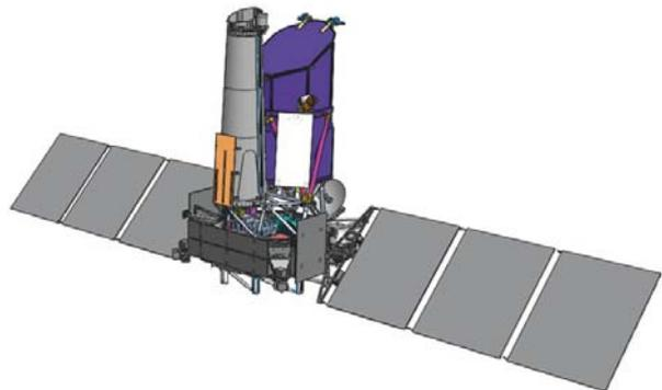
**Fig. 1** Navigator platform with the Russian instrument ART-XC in front and eROSITA (courtesy Lavochkin Association).
